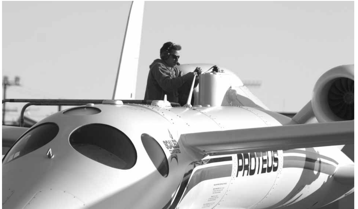
INSTALLING RADIOMETERS on a stabilized platform is John Smith (8227). This keeps the instruments level in spite of small aircraft maneuvers.
