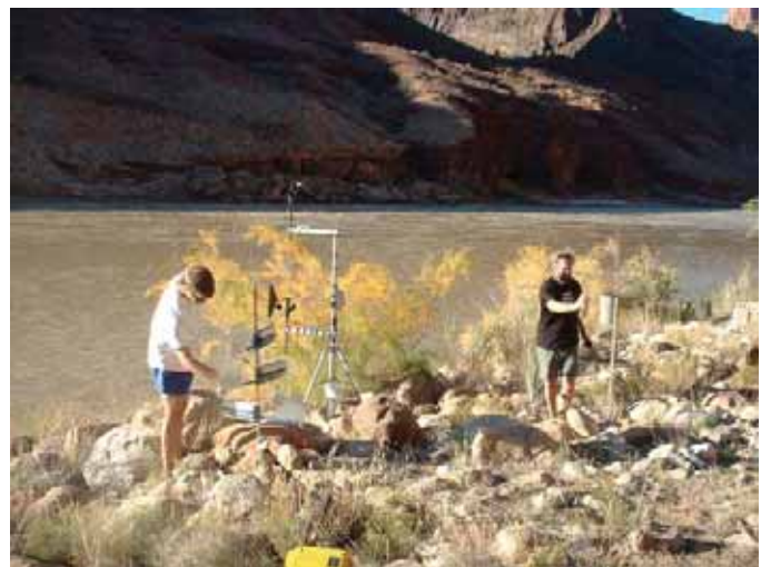
Figure 8. U.S. Geological Survey scientists installing a weather station near RM 65. These devices measure wind velocity and direction at six locations along the Colorado River (photograph by Amy Draut, U.S. Geological Survey).
