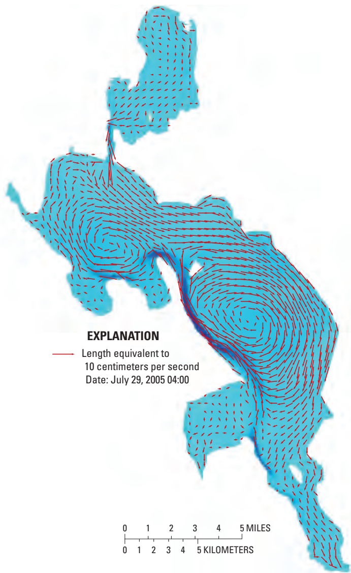
Figure 8. Simulated depth-averaged currents under prevailing (northwest) wind conditions, Upper Klamath Lake, Oregon.
