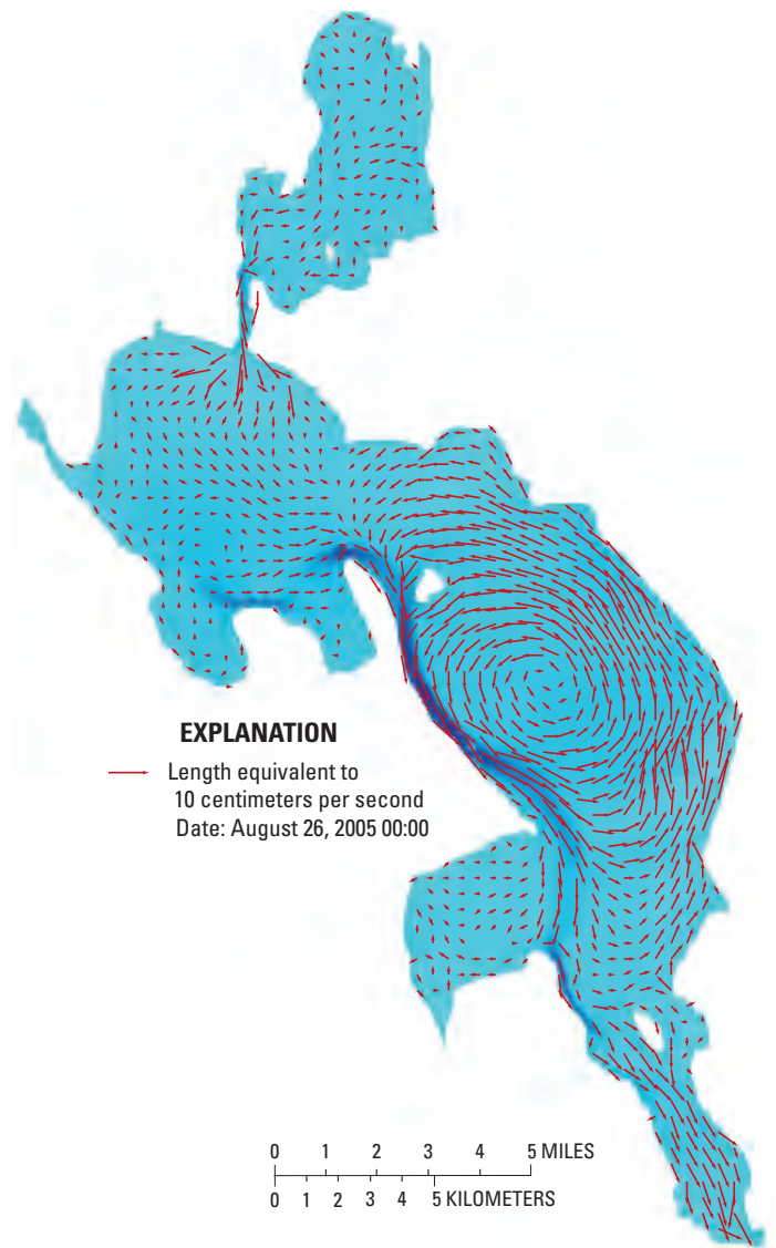
Figure 9. Simulated depth-averaged currents under reversed (southwest) wind conditions, Upper Klamath Lake, Oregon.
