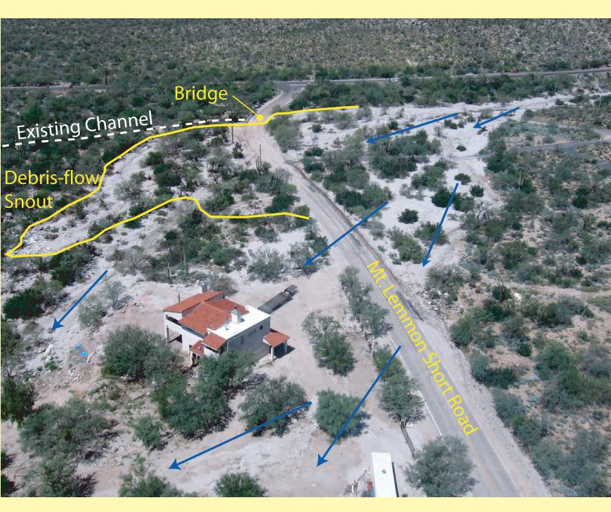
Figure 13. The debris flow in Soldier Canyon filled the existing channel near the Mt. Lemmon Short Road bridge and caused sheet flow
