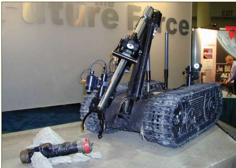
TARDEC's TALON robot with new recoil percussion actuated non-electric (PAN) disrupter mount.
