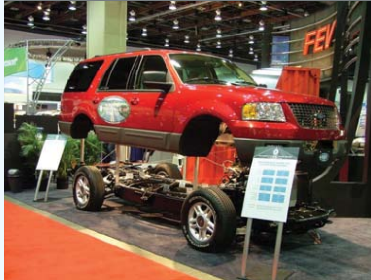
The Ford SUV with hydraulic hybrid technology on display at the Society of Automotive Engineers (SAE) World Congress in 2004.
