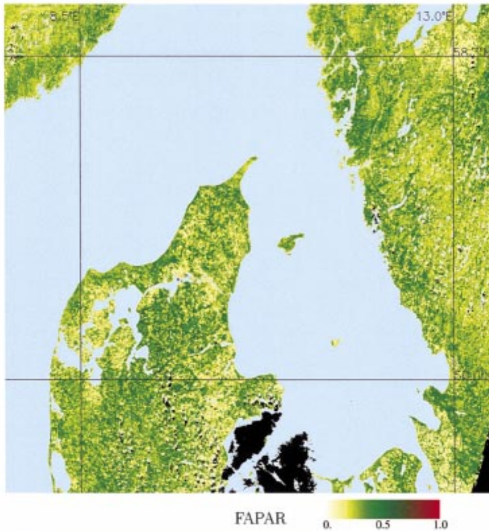
Fig. 9. FAPAR map constructed after 30-day accumulation period using MISR global mode data in September 2000 over Scandinavia. All Terra orbits available over paths 196 to 200 have been considered. The color bar shows the various classes of FAPAR retrieved. The light blue color identifies pixels flagged as “water body and deep shadow” according to spectral criteria defined in Table VI. The black color identifies pixels for which no solution was delivered by the algorithm. The yellow color identifies pixels flagged as “poor fit of RPV”.
