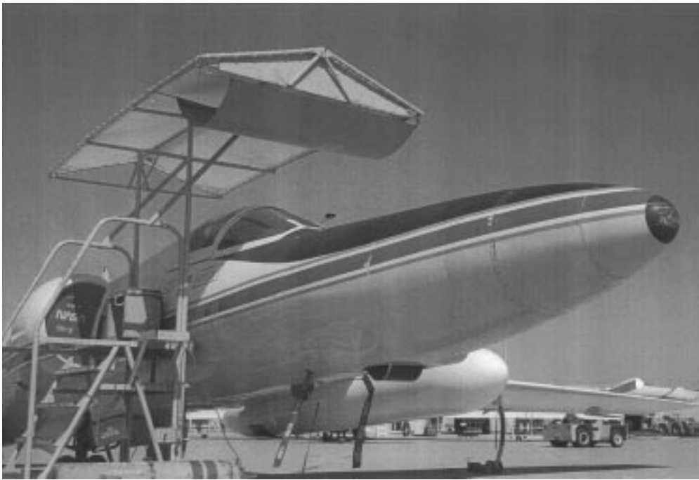
Fig. 3. Rotating drum (which contains the camera) mounted on the bottom of the aircraft just ahead of the cockpit, before an engineering test flight in April 1997.
