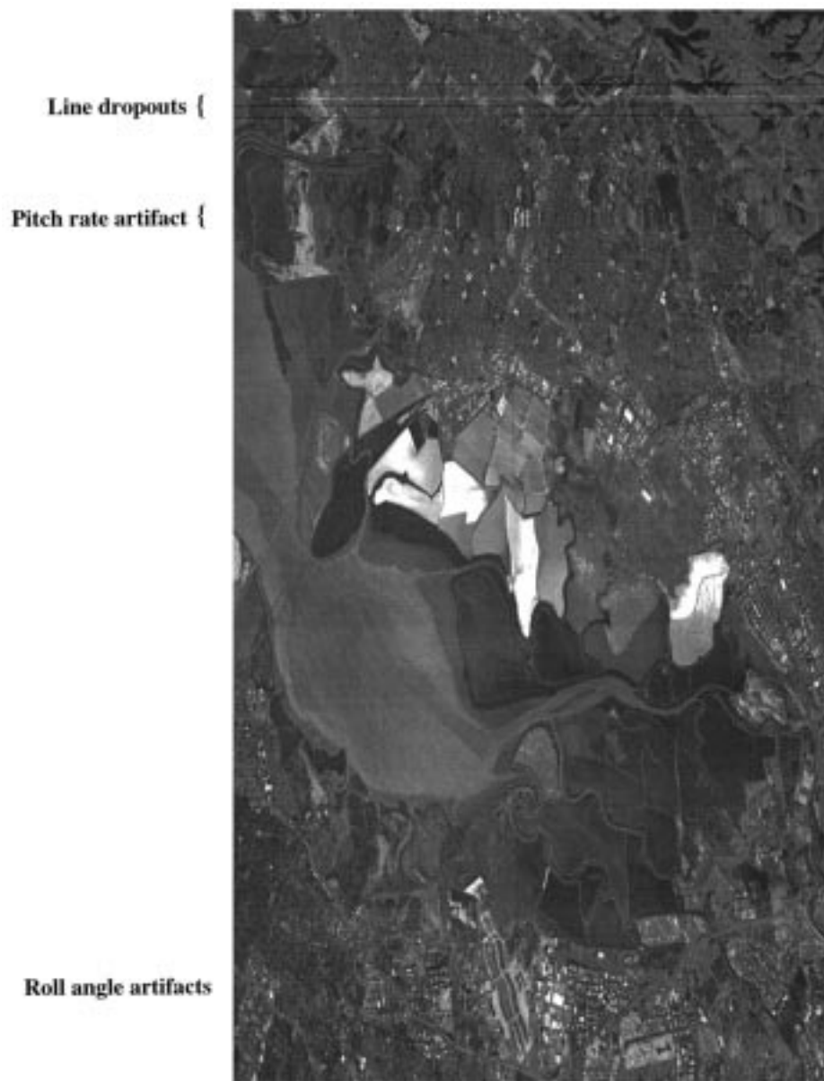
Fig. 5. Red band raw data image at the 60^\circ forward look angle from August 25, 1997.
