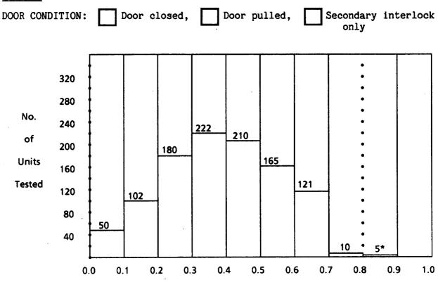
Microwave Leakage (mW/cm<sup>2</sup>) for model family <u>AB</u>
