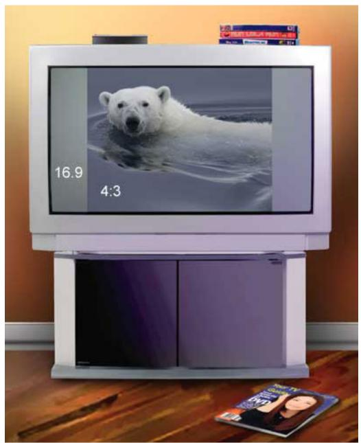
Most HDTVs have a widescreen 16:9 aspect ratio. To accommodate traditional 4:3 aspect ratio broadcasts, most models place gray bars to the sides of the image.
