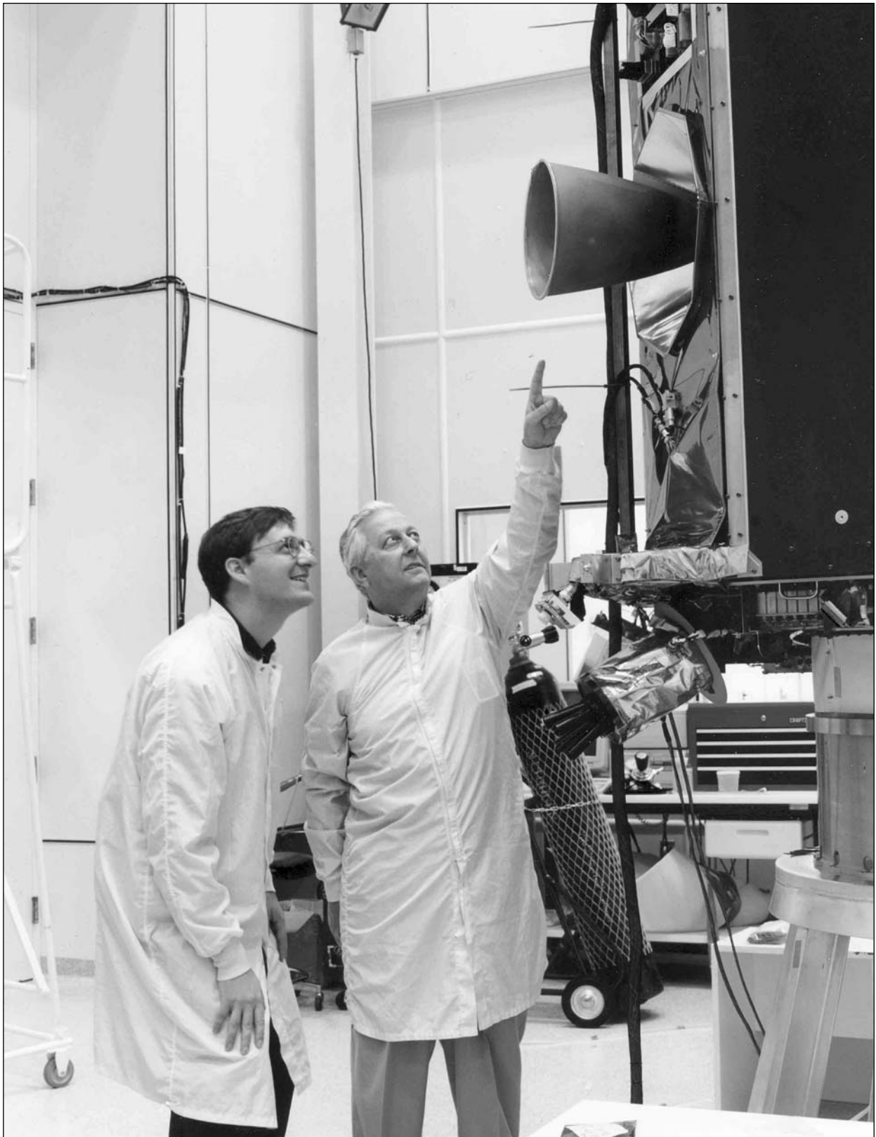
Robert Farquhar (right), Mission Director for the NEAR project, points to the large velocity adjustment thruster on the NEAR spacecraft. Project officials simplified the propulsion system so as to minimize the difficulties of integrating it into the spacecraft.
