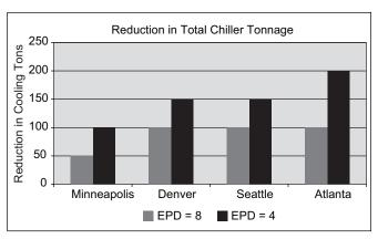
Figure 6. Reduction in chiller tonnage resulting from rightsizing equipment power density (EPD) down from 12 W/sf, to 8 W/sf and 4 W/sf, for different climatic contexts. Based on parametric simulation study of a prototypical 100,000-sf laboratory building [Enermodal and NREL 2003].
