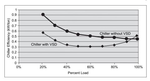
Figure 5. Variable-speed drives are a common strategy for maximizing efficiency at partloads. Data provided by York International Corporation for chillers running at 42°F chilled water supply and 65°F condenser water supply.
