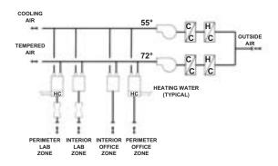
DUAL TEMPERATURE SUPPLY AIR WITH TERMINAL HEATING
