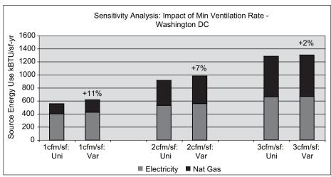
Figure 5. Sensitivity analysis of source energy use intensities for different ventilation rates ("Uni": uniform load simulation; "Var": simulation with load variation). All results are for Washington, DC, climate.
