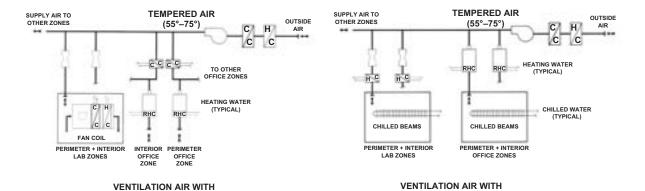
Figure 7. Alternative HVAC systems that minimize reheat energy use caused by load variation between zones.
