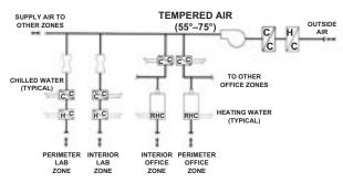
**ZONE COOLING & HEATING COILS**
