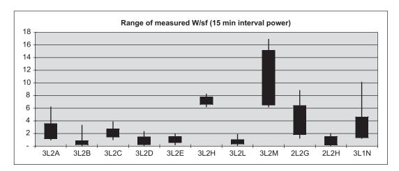
Figure 1. Range of measured 15-min-interval power for various laboratory spaces in a building at UC Davis. The upper and lower ends of the lines represent maximum and minimum, respectively. The upper and lower ends of the boxes represent 99<sup>th</sup> and 1<sup>st</sup> percentiles of the measurements, respectively.
