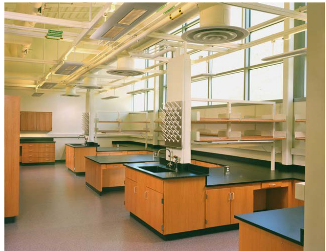
Figure 11: San Mateo County Forensic Laboratory incorporates integrated daylighting and lighting controls, contributing to anticipated energy consumption that is 50% less than mandated by California Title 24. Source: HOK.
