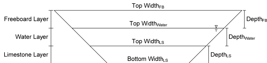
Figure 4-2. End-View of Limestone Bed with Dimensions
