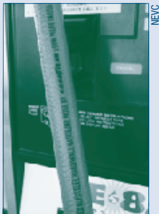
Always use an E85-compatible hose on E85 dispensers.
