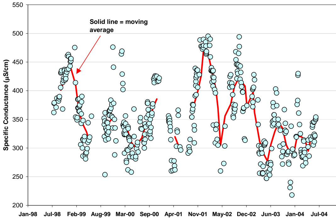
Figure 14. Average daily specific conductance for water samples collected from various sampling sites throughout the distribution system (1998 – 2004). The 3-month running average specific conductance for water in the distribution system is shown for comparison.
