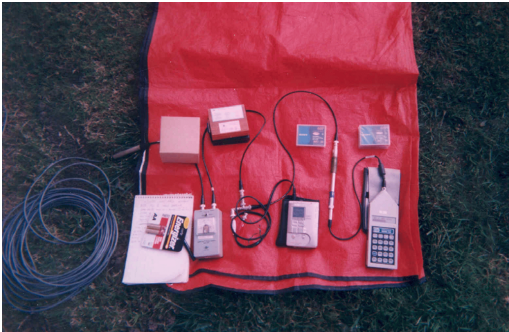
Figure 3. Sound Level Meter and DAT Recorder Attached to Microphone System.
