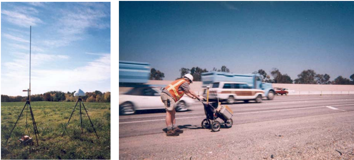
Figure 6. Differential GPS System: Base Station and Roving Unit.
