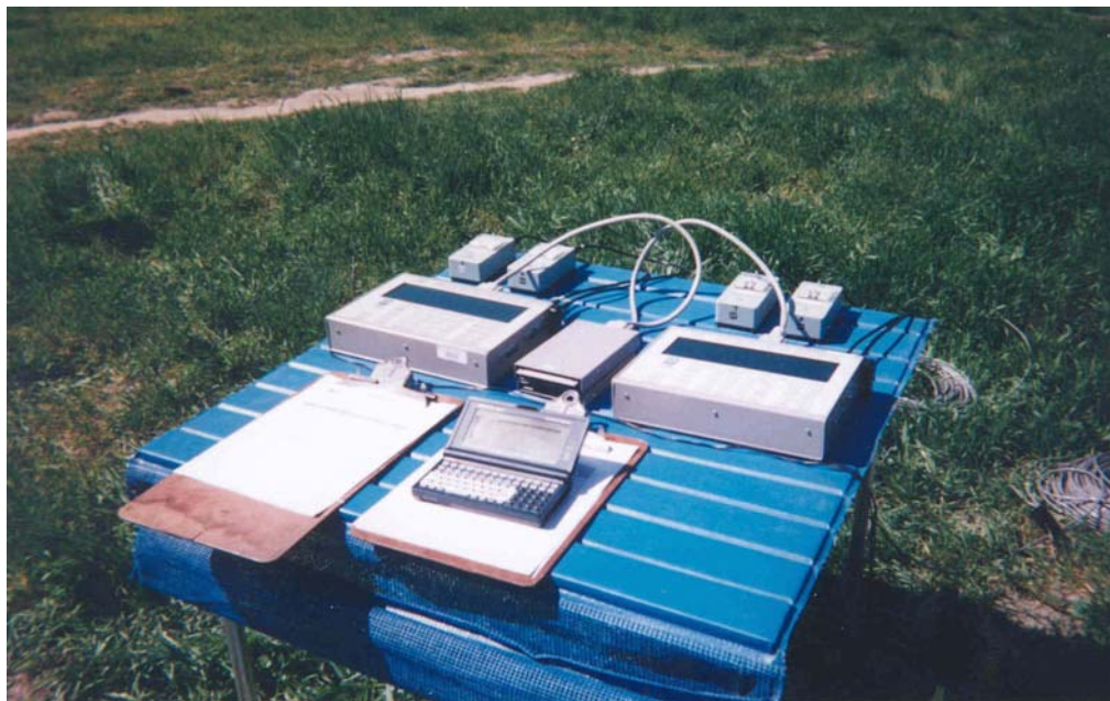
Figure 2. Two Spectrum Analyzers at Acoustic Observer's Station.
