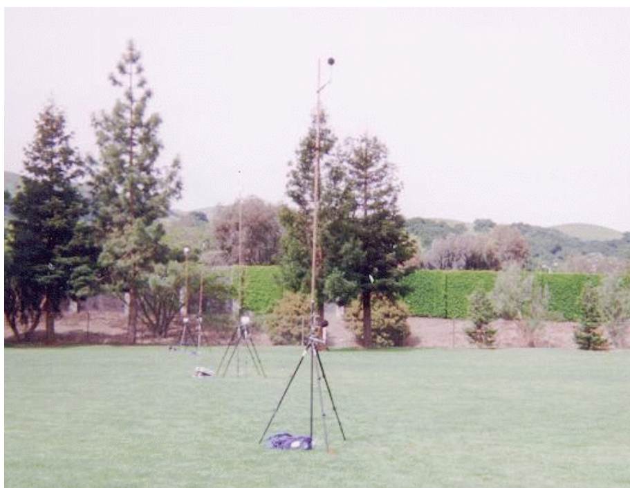
Figure 10. Line of Microphones and Meteorological Systems at Site 12CA.
