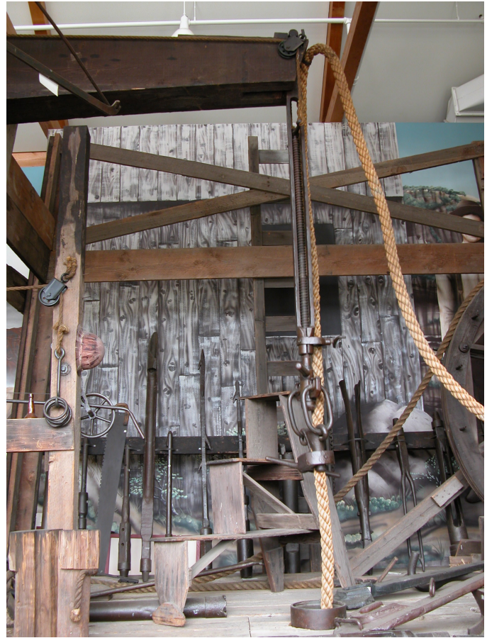
Figure 3.20. View of the cable mechanism used on early steam-powered drilling rigs.
