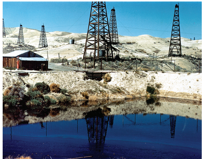
Figure 3.56. Typical oil sump. Location and date are unknown. Photograph courtesy of Don Arnot, West Kern Oil Museum.
