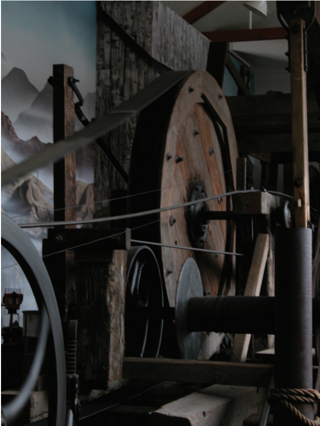
Figure 3.18. Wooden band wheel and belt used in early steam-powered drilling rigs.
