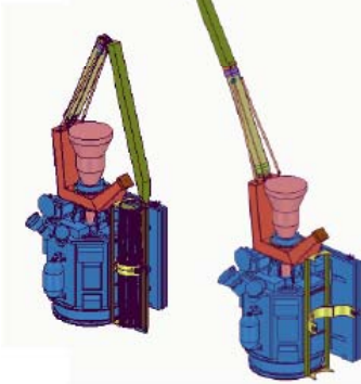
Figure 4. SMAP antenna design options and notional spacecraft depictions incorporating radial rib (top) and perimeter truss (bottom) technologies.
