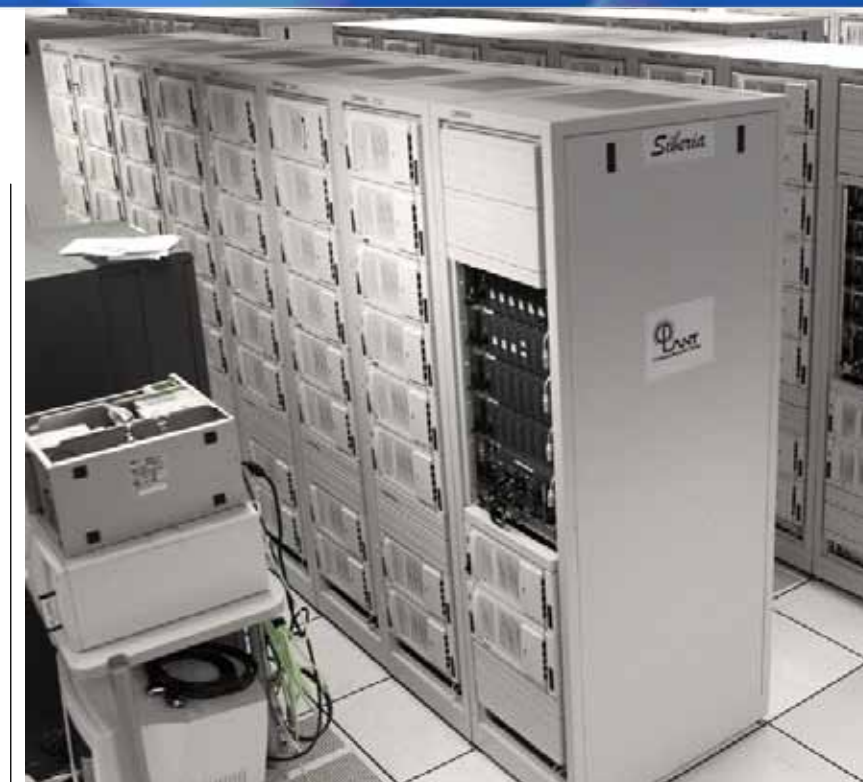
The C Plant Computer, built at Sandia from commodity parts.
