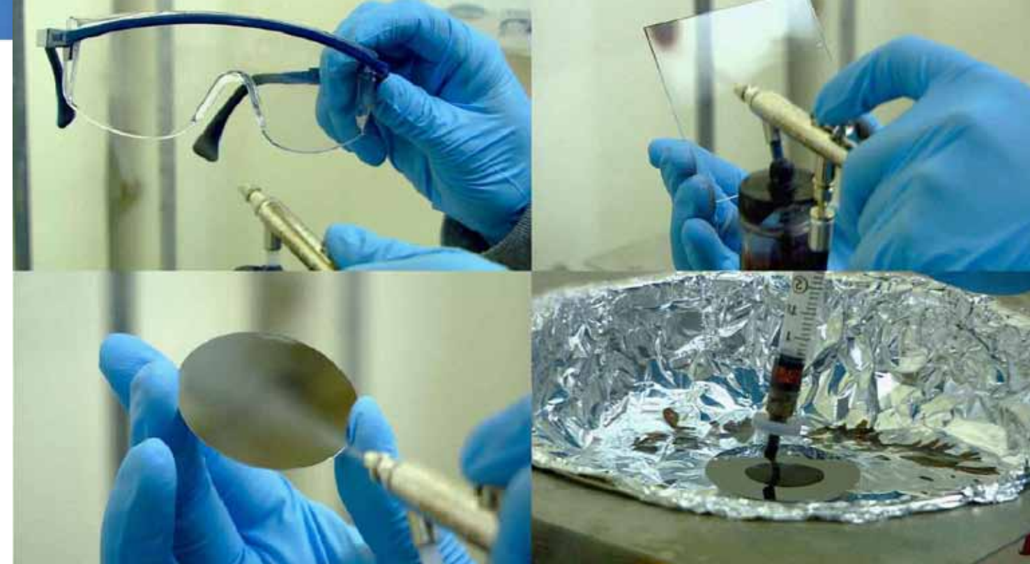
Spray-coating thin films onto a diversity of surfaces is a relatively easy process.
