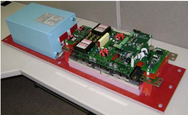
Silicon Power's Standard Building Block for the Solid State Current Limiter
