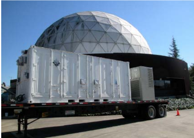
500Kw battery system on DUIT site, San Ramon Ca. 5/2007
