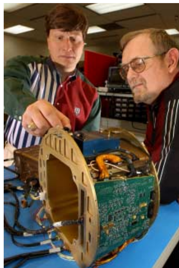
RING OF ELECTRONICS — Mark Beader (left) and Randy Swier (both 2334) examine a Toroidal Electronics Package (TEP), designed at Sandia, that serves as the navigation, guidance, and control system for TACMS-P. (Photo by Randy Montoya)
