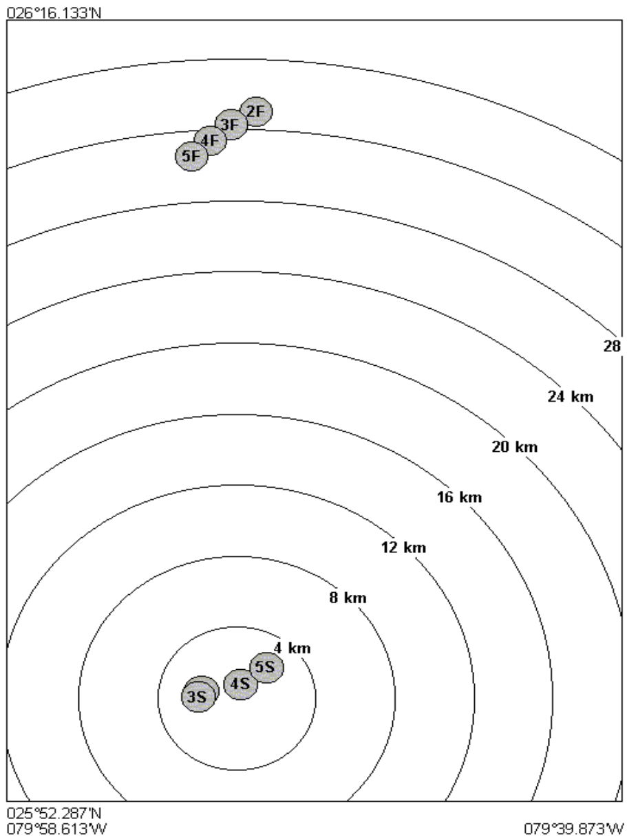
Figure A -1. Explorer Drifter Tracks (S -Start and F -Finish) for Set of Five Drifters Deployed and Recovered during the Miami Plume Tracking Survey.
