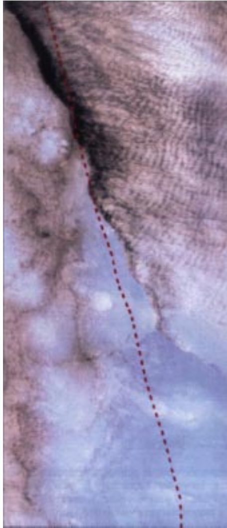
Plate 13.2 A red (2.14 \mu\text{m} ), green (1.62 \mu\text{m} ), and blue (0.66 \mu\text{m} ) composite image of marine stratocumulus clouds in the eastern Atlantic, derived from 2320 scan lines of MODIS Airborne Simulator (MAS) data on June 17, 1992, between 1221:21 and 1227:33 UTC. The dashed line superimposed on this image represents the location of the University of Washington C-131A in situ observations presented in Figure 13.6.
