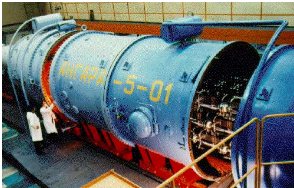
RUSSIAN SCIENTISTS examine one arm of their ANGARA-5-1 pulsed power machine at Kurchatov Institute in Moscow. The device, like Sandia’s Z machine, is exploring z-pinch phenomena.
