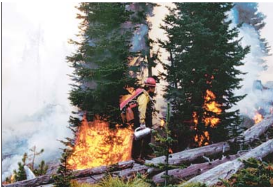
Figure 3.4.1. Bitterroot Hotshot crew member wearing backpack that obtains smoke exposure samples collected within several inches of a worker's face.
