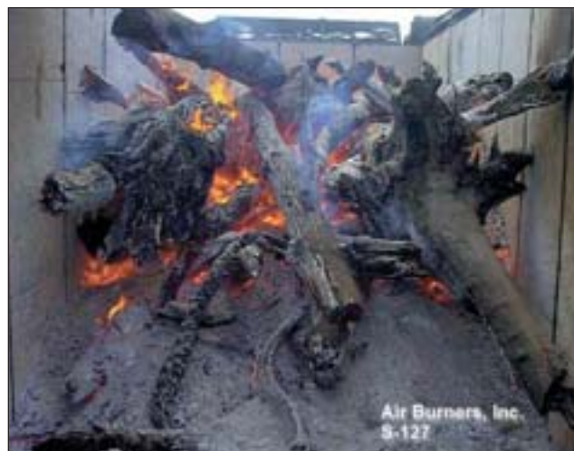
Figure 8.8. Air curtain incinerators result in very hot and efficient fires that produce little smoke.
