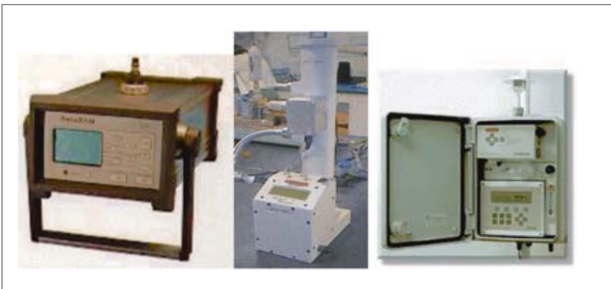
Figure 10.1. Three of the nephelometers tested during the Trent and others (2000) study include the MIE DataRam, the Radiance Research nephelometer, and the Met One GT-640.
