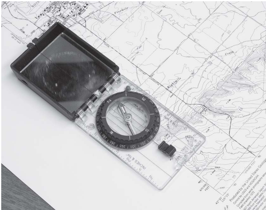
Figure 6-2. Orienting a map with compass.
