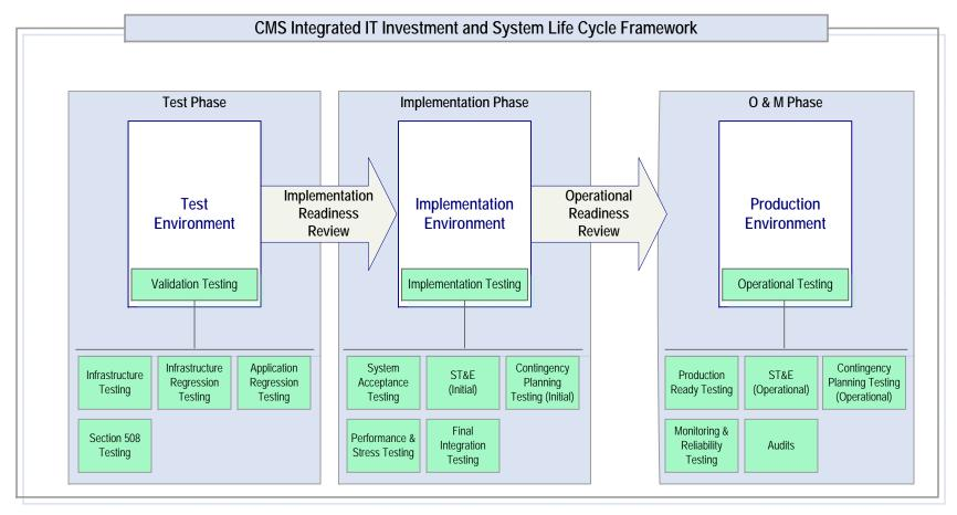
**Figure 2: Infrastructure Testing Functions**
