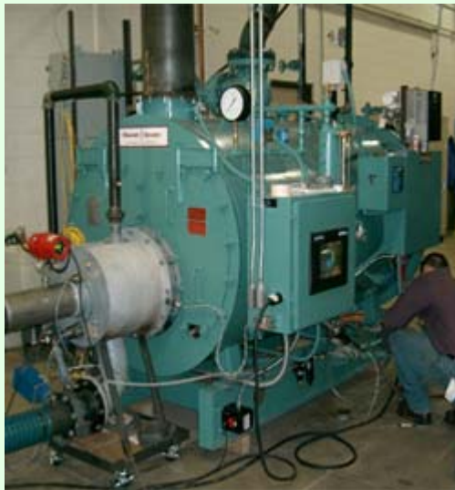
Figure 5.5 Laboratory Prototype Boiler (Rabovister and Knight, 2005)
