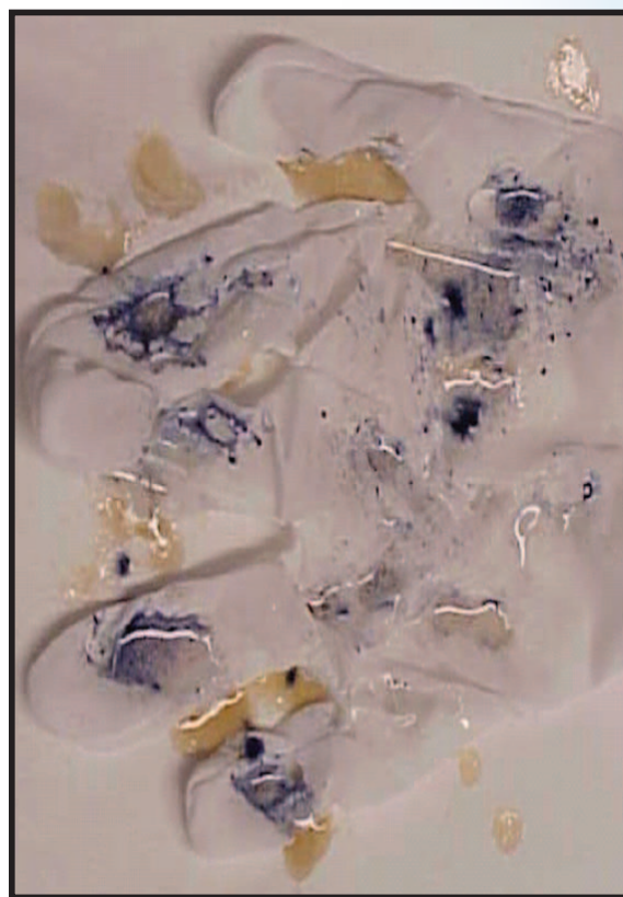
Colored spots on inspector's glove indicate presence of explosives.
