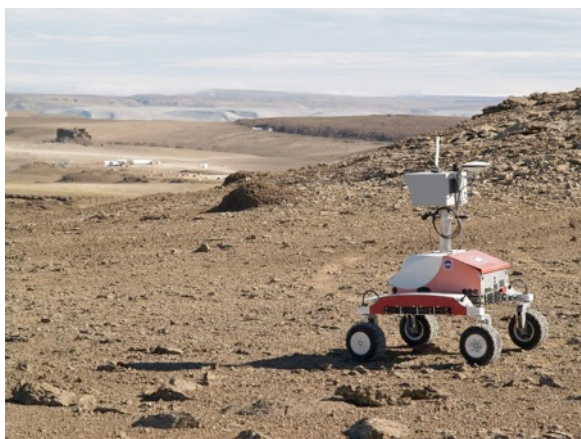
Figure 1. K10 “Red” with a mast-mounted Optech ILRIS-3D lidar at Haughton Crater.
