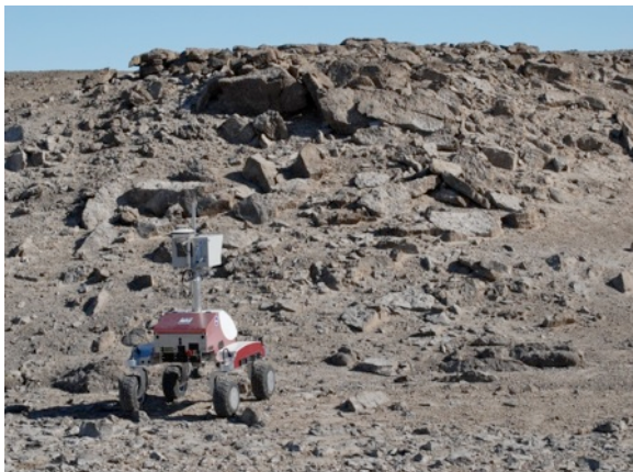
Figure 8. K10 Red scanning a steep and rocky slope during lidar survey.
