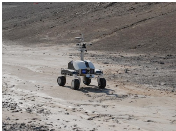
Figure 2. K10 “Black” with the CRUX GPR (mounted under chassis) at Haughton Crater.
