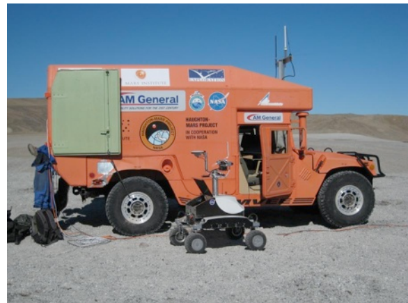
Figure 5. HMMWV used to simulate a “pressurized rover” for Drill Hill survey.
