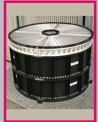
The 5 X-Ray Telescopes (XRT) will focus x rays onto the XIS and XRS detectors.
