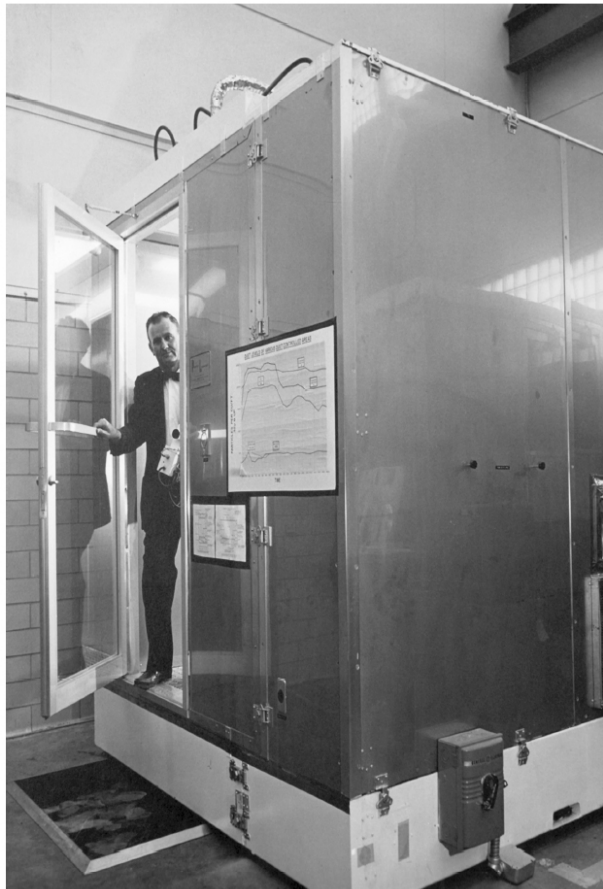
Laminar-flow Clean Room: Willis Whitfield stands in the doorway of his prototype of the Ultra-Clean or Laminar-flow Clean Room, which he developed to enable the manufacture of close-tolerance parts. The new design significantly improved existing clean room technology and transformed manufacturing of microelectronics and pharmaceuticals, surgical environments, and food production hygiene.
