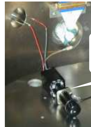
Light-tight PMT assembly in vacuum chamber for corona test
