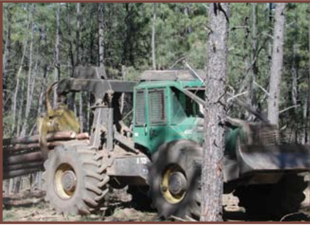
Grapple skidder operating on restoration project.
