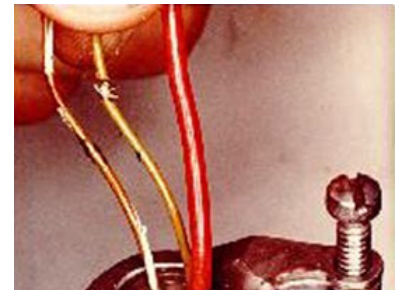
Figure 5. Wire failure mechanisms: mechanical.
