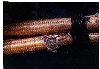
Figure 2. Wire failure mechanisms: chemical.
