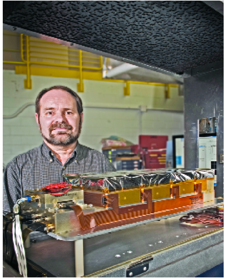
Technologist Scott Barthelmy believes this instrument prototype would be useful for detecting nuclear material hidden in shipping containers and trains. He developed it using leftover components from Goddard's Burst Alert Telescope.
