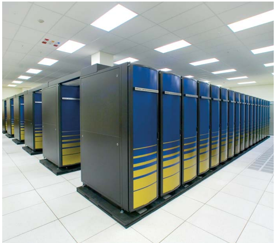
FIGURE 1. NERSC's Cray XT4 supercomputer, when complete, will deliver sustained performance of at least 16 teraflop/s.
