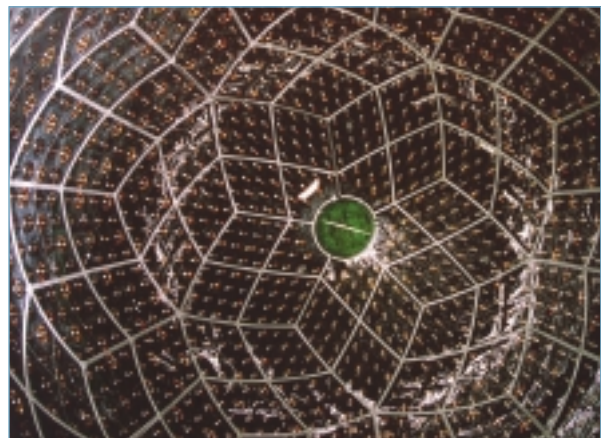
FIGURE 1 Looking up at KamLAND's photomultipliers. When a neutrino collides with a proton in the liquid scintillator, a flash of light is emitted that is detected by the photomultipliers and converted into an electronic signal for computer analysis.
