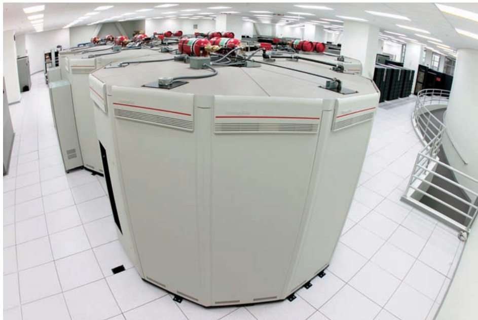
Cost Efficient Archive: HPSS at NERSC archives petabytes of data on systems consisting of spinning disks and tapes.
