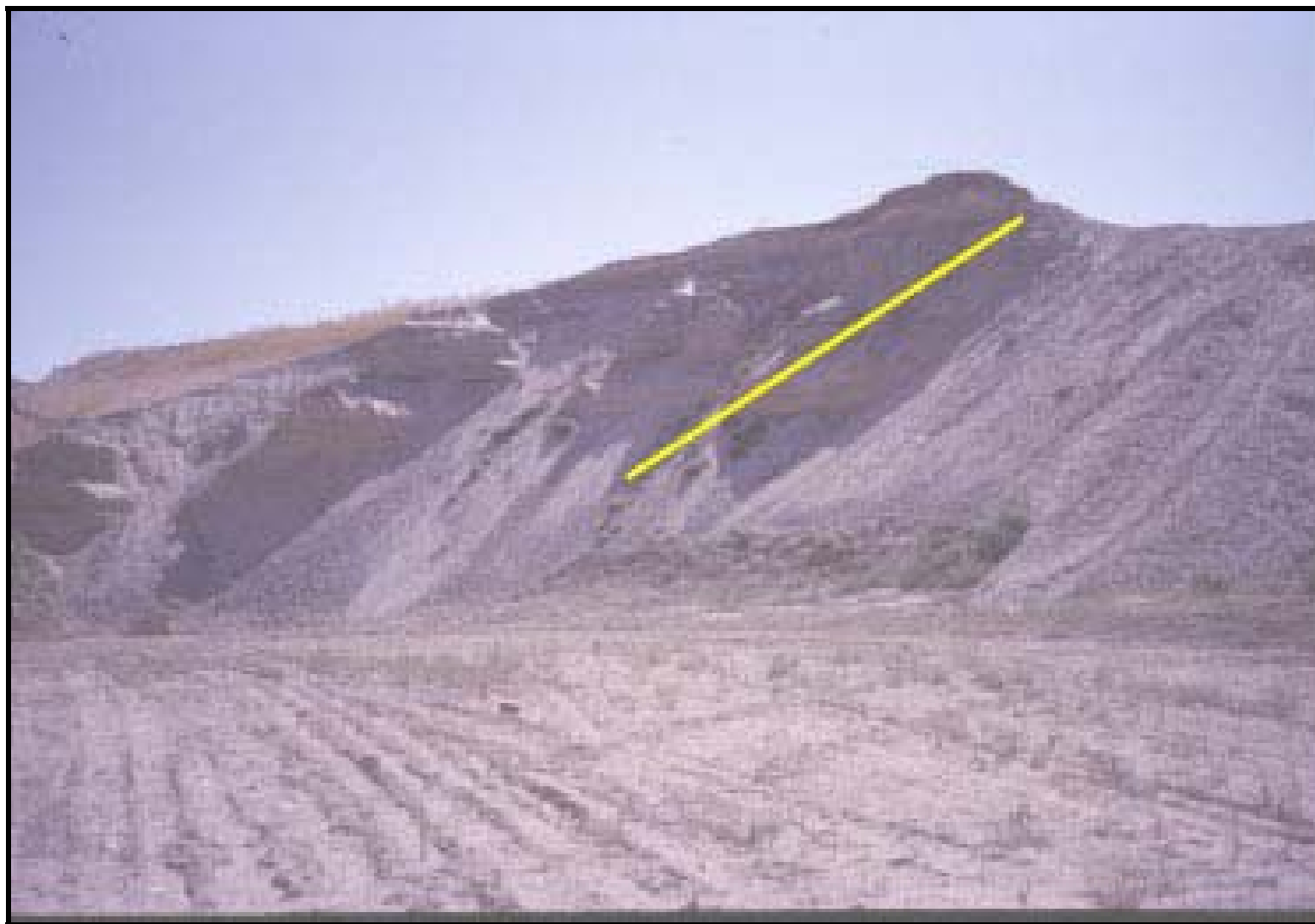
Figure 2. Photograph of U.S. Geological Survey sample site GS-99.02, Ada County Bureau of Land Management Free Use Permit site (AD-5003) on Tenmile terrace. Sample was collected by continuous channel method along the path displayed by the yellow line.
