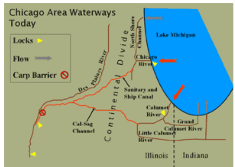
Chicago Area waterways map showing location of carp barrier (Illustration courtesy of Phil Moy, University of Wisconsin Sea Grant Institute)
