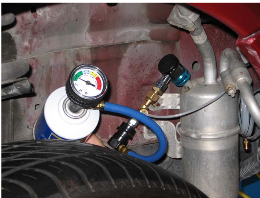
Figure 2: Small Can with Charge Kit and Adapter Installed on the Ford Focus Accumulator Service Port
