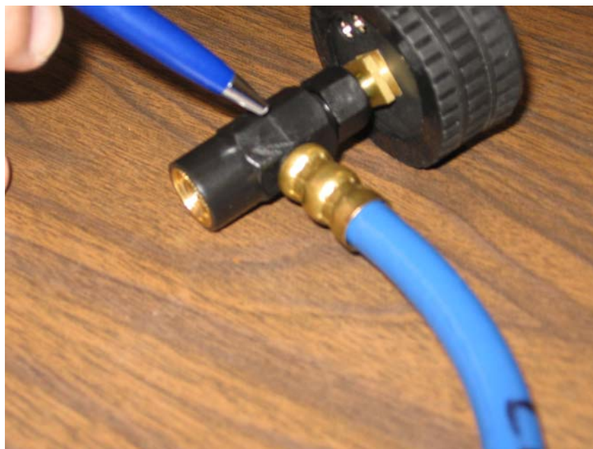
Figure 9: Charge Kit Leak Locations b. Hose Leak at Can Tap
