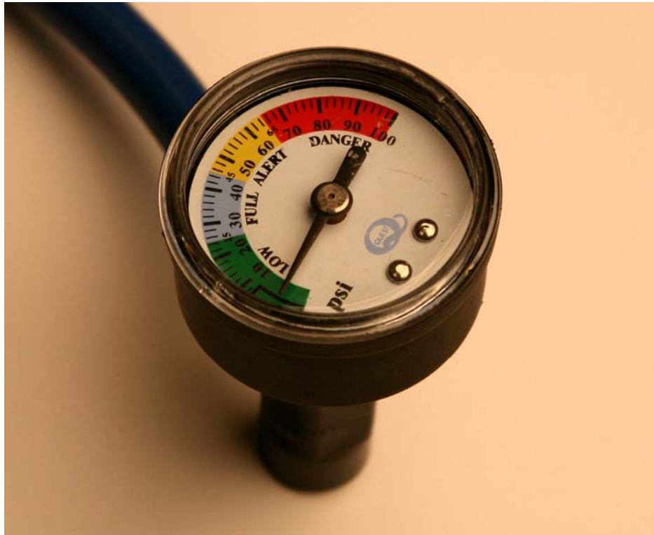
Figure 8: Example of Charge Kit Pressure Gauge with System Charge Ranges
