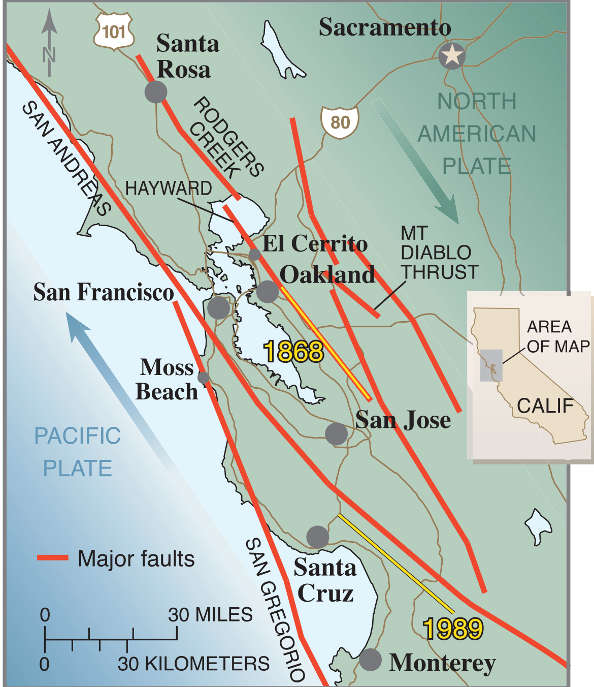
Figure 2.1. Major faults of the San Francisco Bay Region. Arrows show the mostly strike-slip sense of tectonic plate motion accommodated by earthquakes and aseismic creep on SFBR faults. Yellow lines indicate extent of rupture in the 1868 M \sim 6.8 earthquake on the southern Hayward faults and that in the 1989 M 6.9 Loma Prieta earthquake near the San Andreas fault northeast of Monterey Bay.
