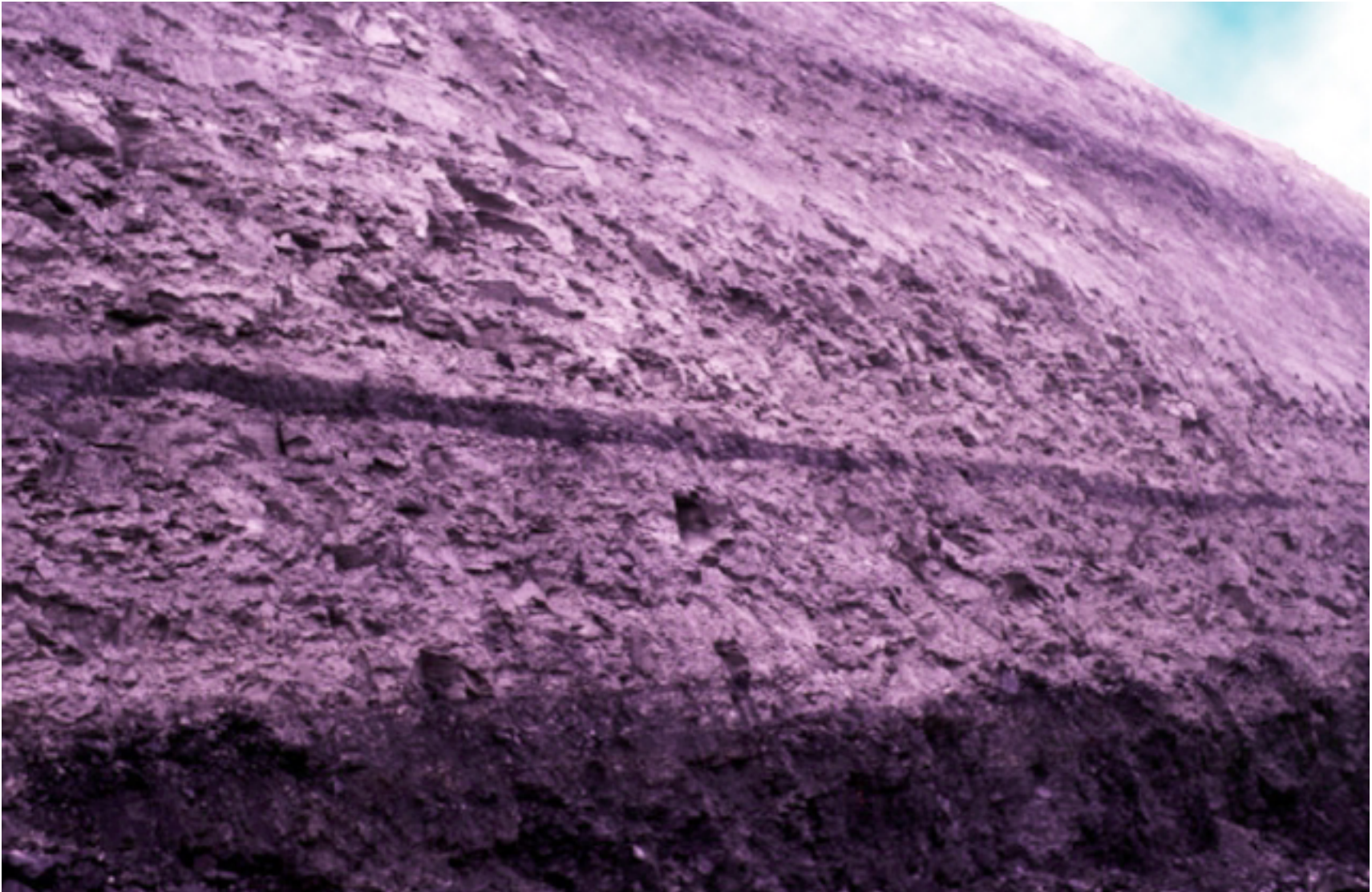
Figure WF-8. The Beulah-Zap coal zone in the Freedom mine is overlain by a thin rider coal and mudstone. Photograph by R.M. Flores.
