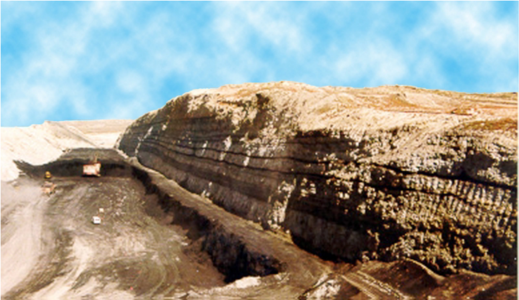
Figure GS-10. Highwall in the Black Butte coal mine showing stacked, fining-upward fluvial channel sandstone and overbank deposits. Photograph by R.M. Flores.
