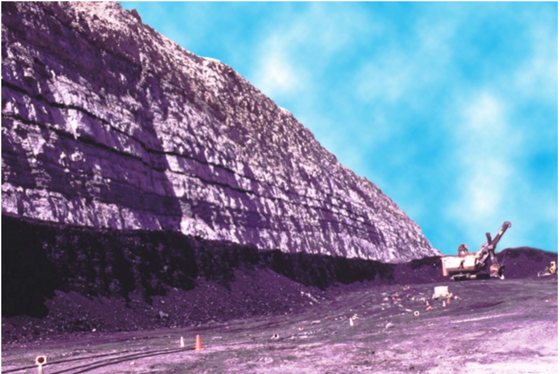
Figure GS-7. Tabular-shaped crevasse splay sandstone beds are interbedded with siltstone, mudstone, coal, and carbonaceous shale. These deposits are exposed along the mine highwall of the Jim Bridger coal mine. Photograph by R.M. Flores.
