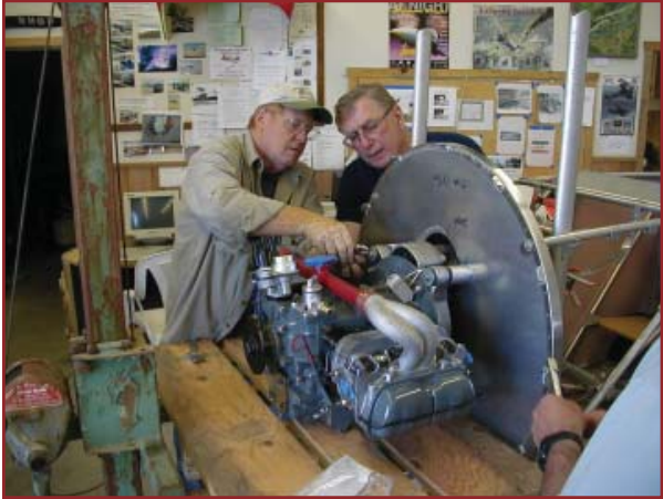
Bill McMichael (left) and a volunteer fine tune the 60 horsepower Volkswagen 1835 c.c. engine that allows the aircraft to cruise at nearly 80 m.p.h.
