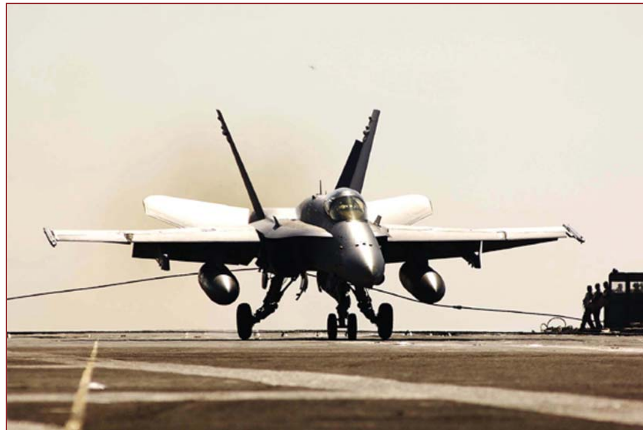
An F/A-18C aircraft makes an arrested landing on a flight deck of a U.S. aircraft carrier.
