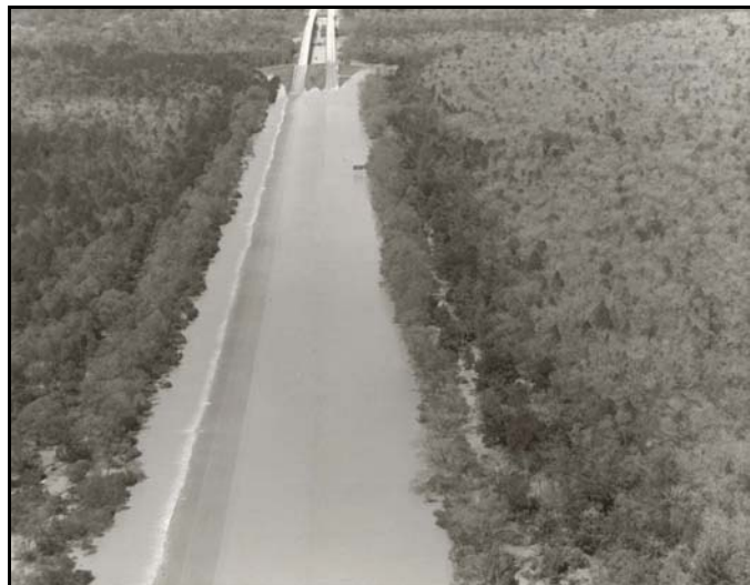
Figure 3-9. Weir flow over roadway embankments is modeled using an empirical formula that connects finite element networks on the upstream and downstream sides of the embankments.
