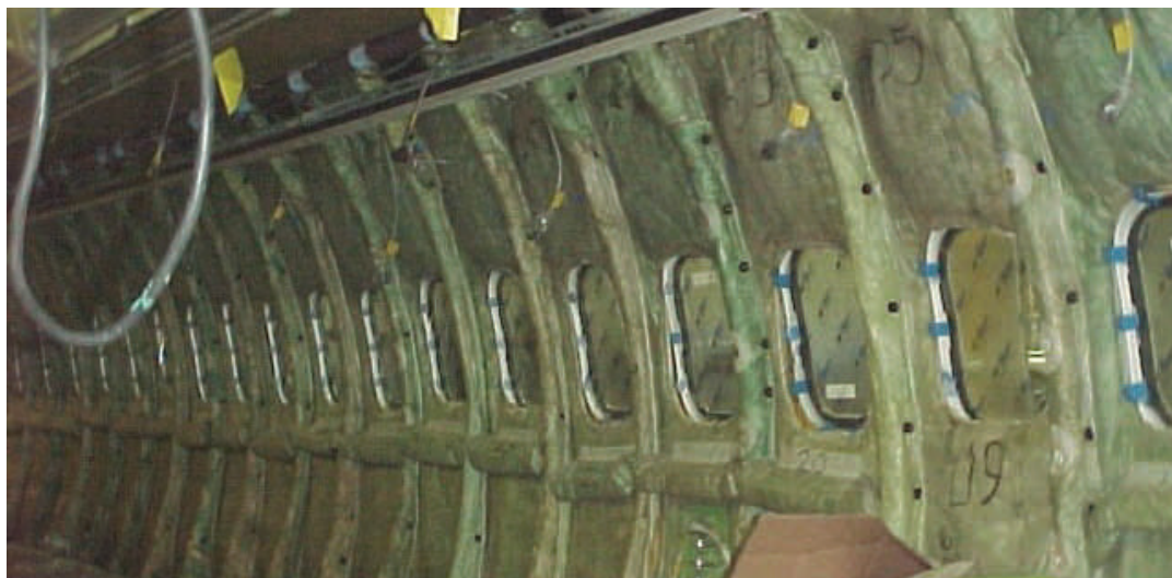
AN-26 is used extensively behind the sidewalls of the main cabin.
