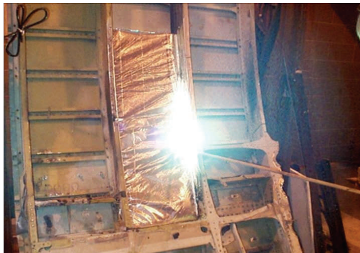
Arc testing conducted on MPET.
